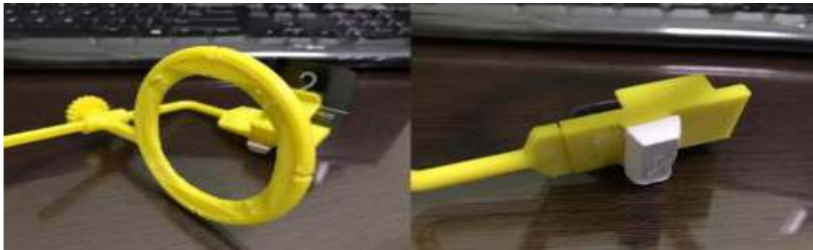
Figure 2. One set of holder + silicone lining on the bottom of the holder
