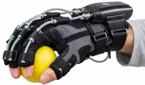
Figure 2. A robotic glove used for stroke rehabilitation.
